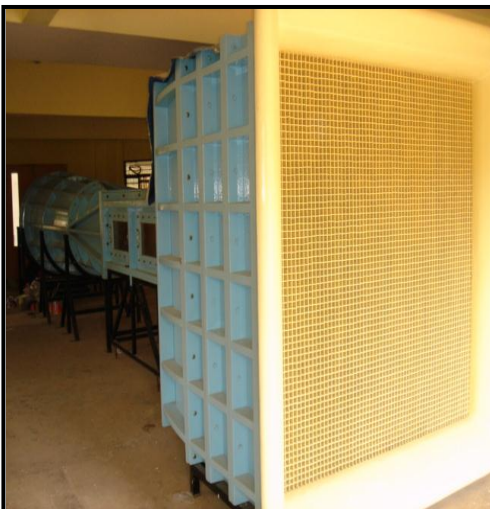
KBN COLLEGE OF ENGINEERING, GULBURAGA. TEST SECTION: 0.6X0.6X2 mts, 50 m/sec
