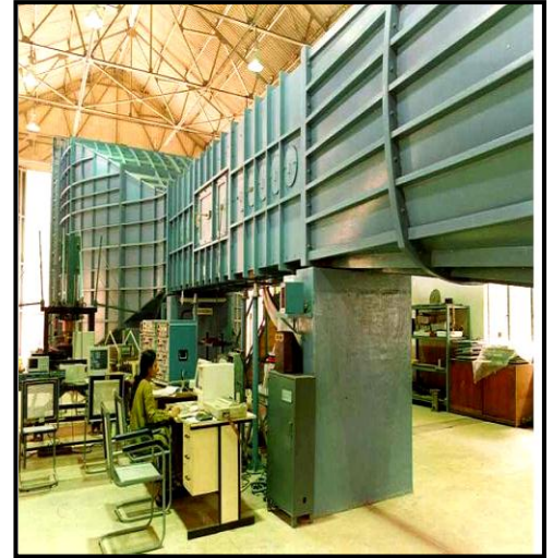
NAL, BANGALORE. TEST SECTION: 1.5x1.5x4 mts, 50 m/sec
