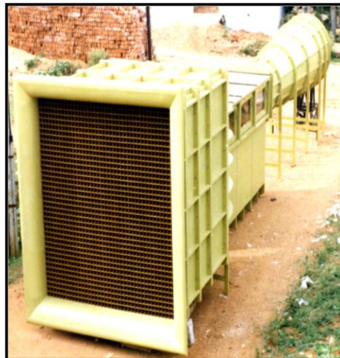
KUWAIT WIND TUNNEL. TEST SECTION: 0.3x0.3x1.2 mts, 50 m/sec
