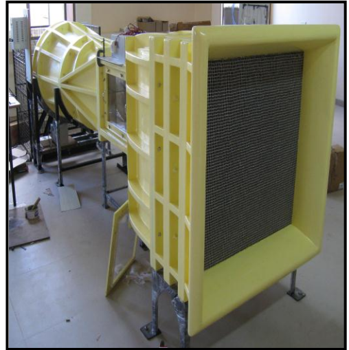
IIST, THIRUVANATHAPURAM. TEST SECTION: 0.3X0.3X0.6 mts, 40 m/sec
