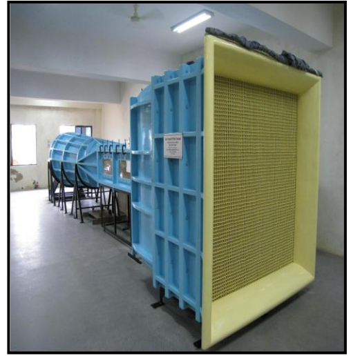
Sri Bhagawan Mahaveer Jain college of Engg Bangalore. TEST SECTION: 0.6X0.6X2 mts, 45 m/sec
