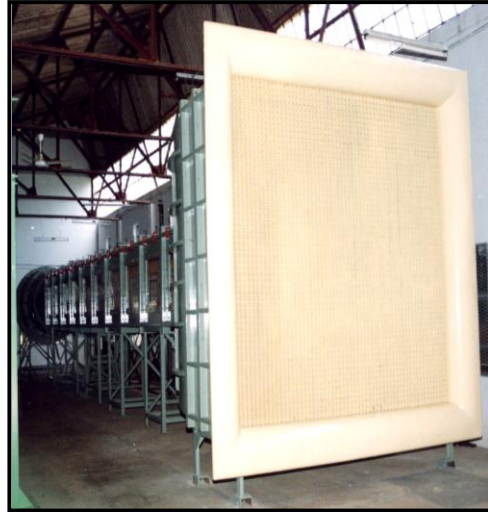
PES, MANDYA. TEST SECTION: 1.2x1.2x7 mts, 25 m/sec
