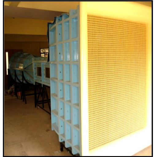
MVJ COLLEGE, BANGALORE TEST SECTION: 0.6x0.6x2 mts, 40m/sec
