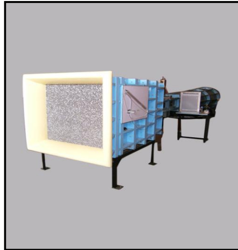
CAREER INSTITUTE OF TECHNOLOGY & MANAGEMENT, FARIDABAD. TEST SECTION: 0.3x0.3x1 mts, 45 M/SEC
