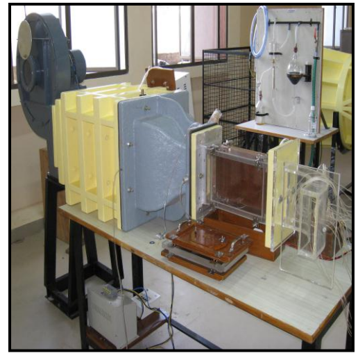
IIST, THIRUVANATHAPURAM MODULAR AIR FLOW BENCH TEST SECTION: 0.15X0.05X0.3 mts, 30 m/sec
