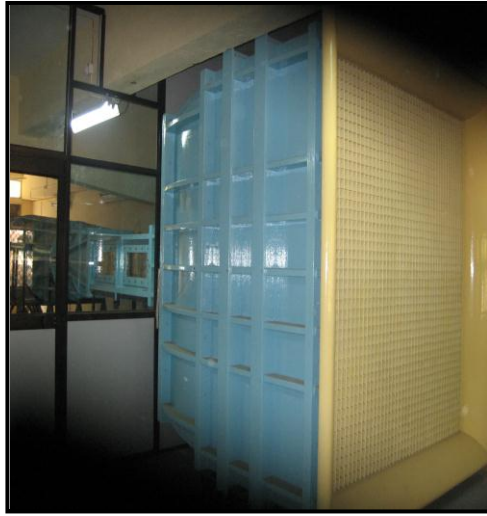
IIT, BOMBAY. TEST SECTION: 0.6X0.6X2 mts, 50 m/sec
