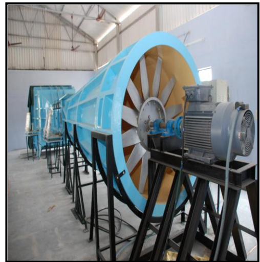
AMRITHA VISHWA VIDYAPEETAM, COIMBATORE. TEST SECTION: 0.6X0.9X2 mts, 45 m/sec
